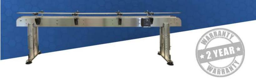
The traditional stainless steel SC series conveyor comes standard with a 4.5" Acetal chain in lengths of 5,10,15 and 20 feet, with custom lengths available. The SC series conveyors are variable speed gear driven and constructed of heavy duty 304 stainless steel.
