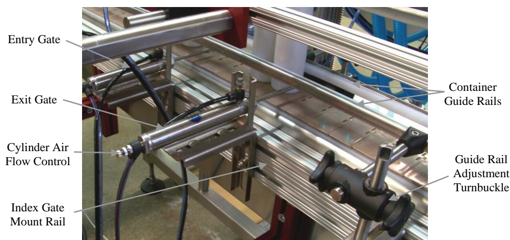
Figure 4-4 Guide Rails and Indexing Gates
